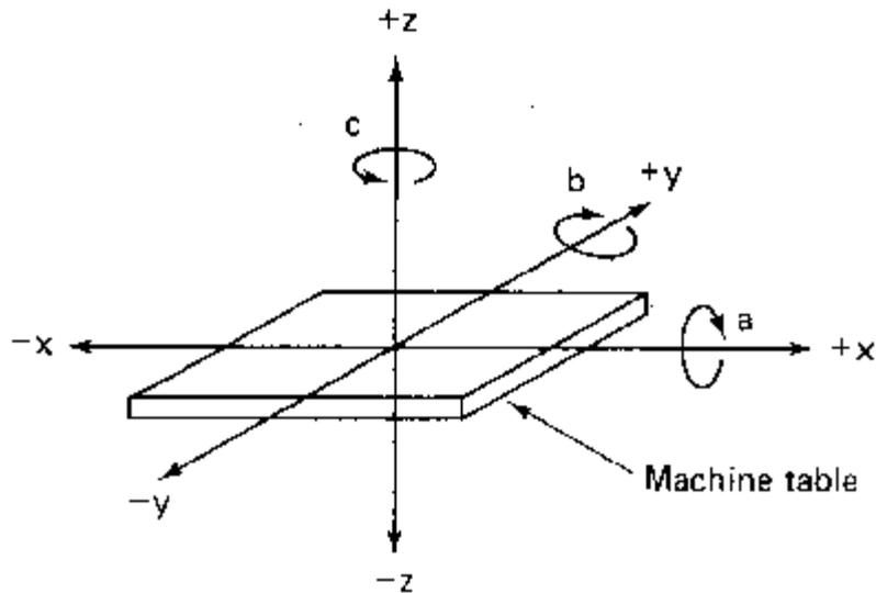
Two axes  $x$  and  $y$  are defined in the plane of the table. The  $z$  axis is defined in the plane perpendicular to the table and the movement in the  $z$  direction is controlled by the vertical motion of the spindle. The positive and negative directions of motion of the cutting tools are relative to the table along these axes. NC drill presses are classified as other two axis or the three axis machines, depending on whether or not they have the capability to control the  $z$ -axis.
