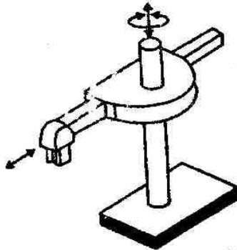
**Fig. Cylindrical configuration.**
