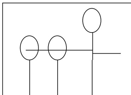
In this system, the positions are indicated from a fixed zero point or reference point or origin. Here all the tool positions i.e. the center of the hole circles, are marked with references to a fixed zero point. In this case the reference or zero point is left hand bottom corner of the work piece and all the distances are given from this point.
