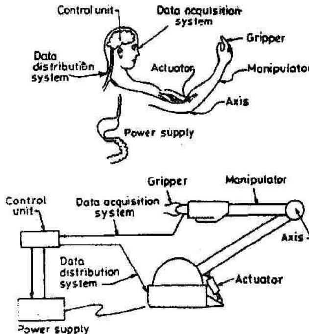
**Fig. Human and Robotic Manipulator systems**
