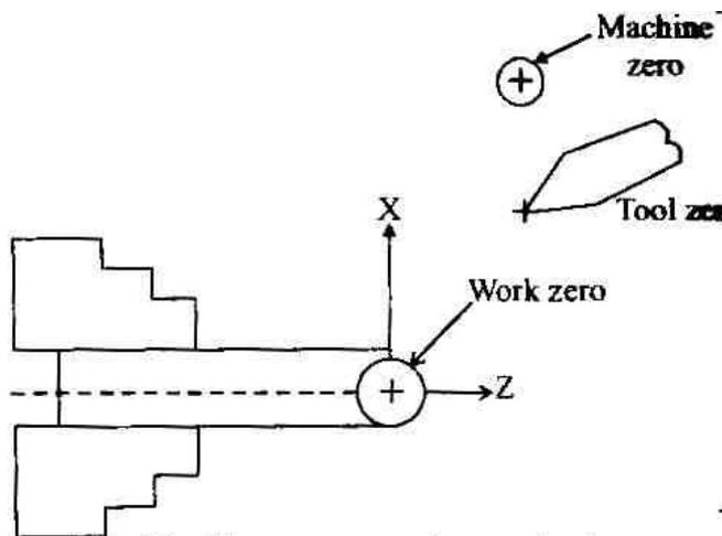
Fig. Machine zero, work zero, tool zero
