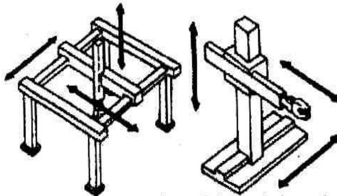
**Fig. Two implementations of the cartesian robot configuration.**
