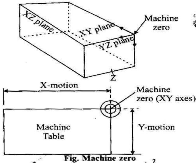
Fig. Machine zero
