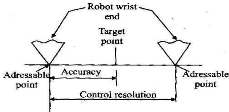
**(Fig : 1 - Accuracy in 2-D frame, without mechanical inaccuracy consideration)**
