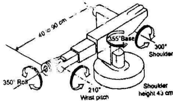
**Fig. Range of motion of spherical coordinate robot.**
