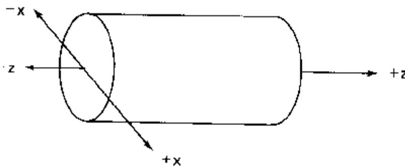
**FIGURE 7.4** The  $x$ - and  $z$ -axes in NC turning.
