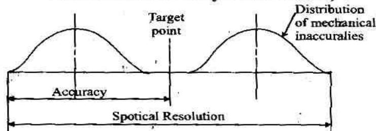
**(Fig : 2 - Accuracy and spatial resolution in which mechanical inaccuracies are represented by a statistical distribution)**
