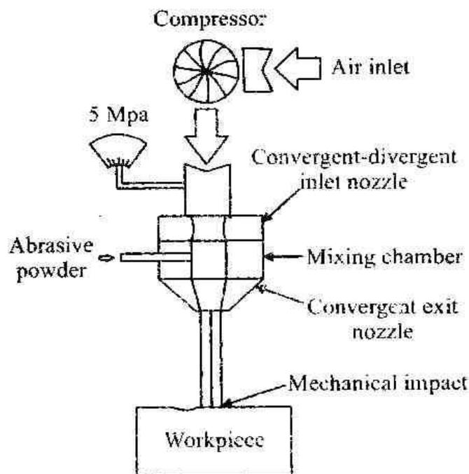
The abrasives generally employed are aluminum oxide., silicon carbide, glass powder or specially prepared sodium bicarbonate. The average particle sizes vary from 10 to 50 microns. Larger sizes are used for rapid removal rate while smaller sizes are used for good surface finish and precision work. In addition to the above abrasives dolomite (calcium magnesium carbonate) of
