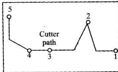
The PTP systems are simplest machine tool control systems. Most suitable for drilling, boring, tapping, punch presses, jig boring machines etc.
