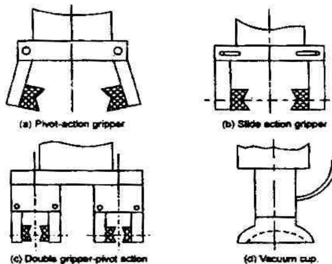
**Fig. Simple gripper designs**
