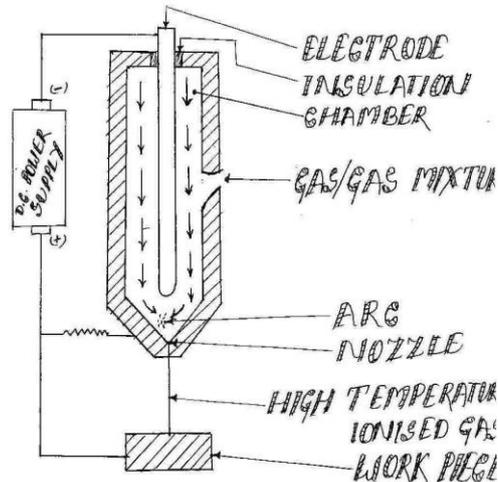
When a gas is heated above 5500°C it is partially ionized and exists in form of mixtures of positively charged ions, neutral atoms and free electrons this mixture is known as plasma.
