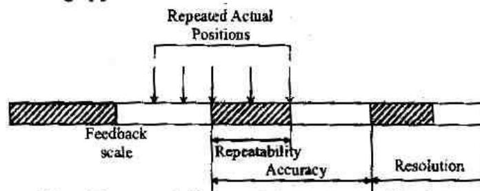
**Fig : Repeatability and Accuracy of Robot**
