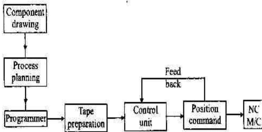
**The main elements of a NC machine tool are :**
