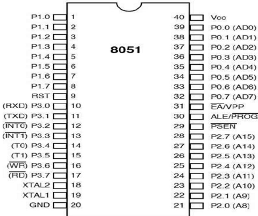
**V<sub>cc</sub> (Pin-40) :-** It is a +5V supply voltage pin.
