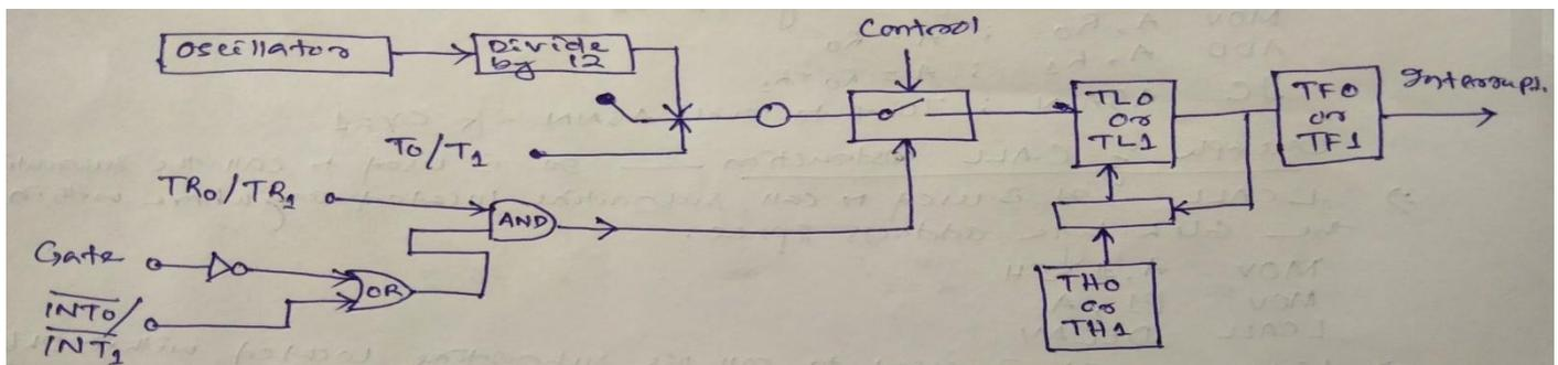
This mode is same for both Timer/counter- 0 or 1. In this mode, T/C register TL<sub>0</sub> or TL<sub>1</sub> is made an 8-bit counter with automatic reload. The overflow from TL<sub>0</sub>/TL<sub>1</sub> sets TF<sub>0</sub>/TF<sub>1</sub> and it also reloads TL<sub>0</sub>/TL<sub>1</sub> with contents of TH<sub>0</sub>/TH<sub>1</sub> which preset by software.
