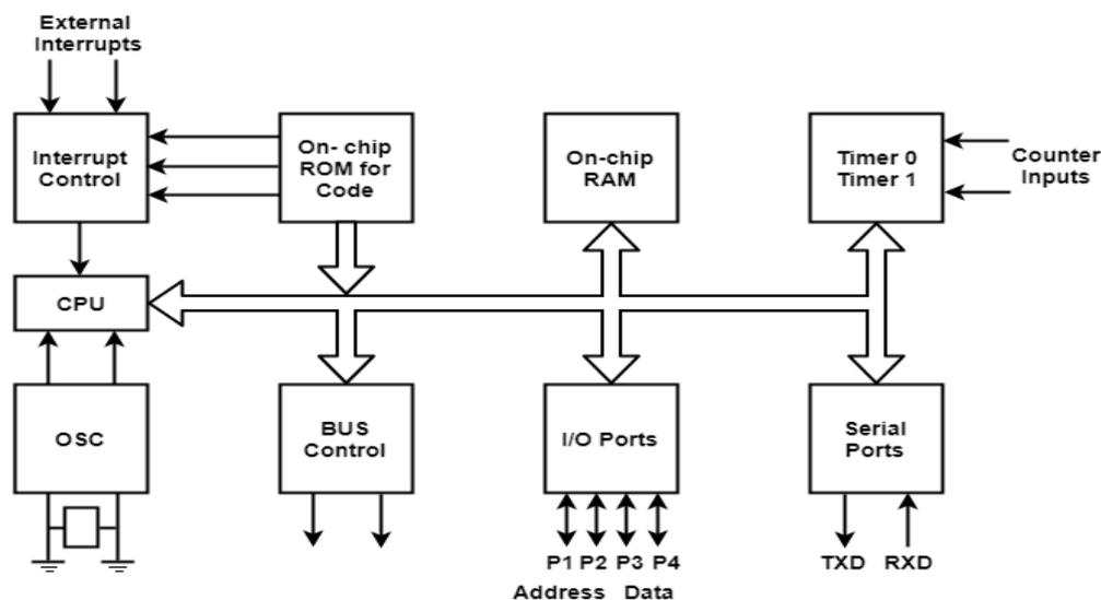
**CPU:-** MCS-51/8051 consists of 8-bit ALU with associated registers like A, B, PSW, SP, the 16-bit PC and DPTR register. The ALU perform arithmetic and logic operation on 8-bit operand.
