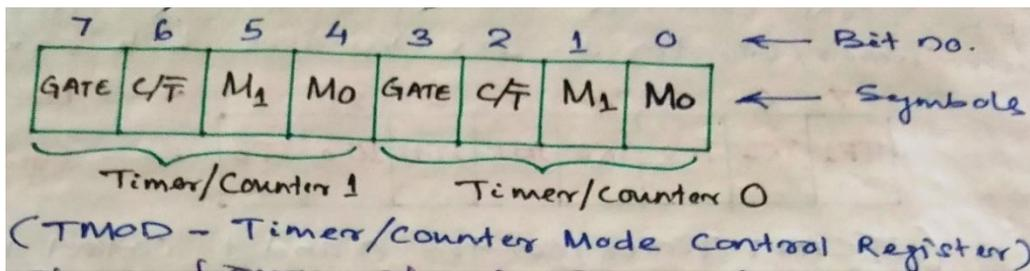
The above figure shows the various bits of TMOD register.
