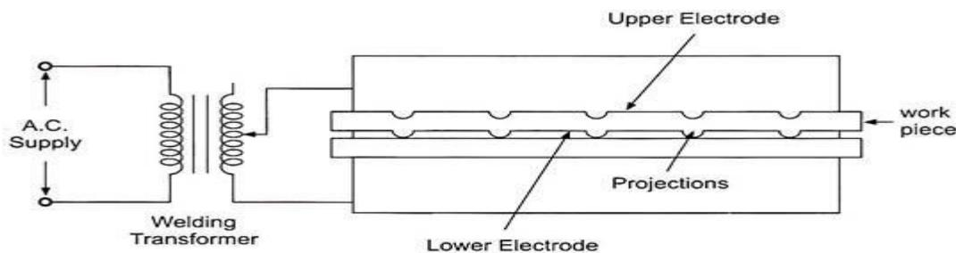
Fig. 4.6 Principle of Projection Welding
