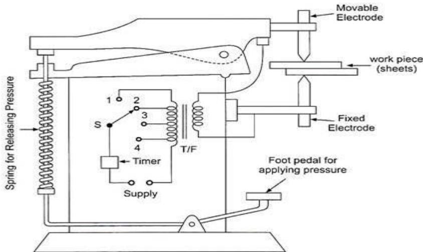
Fig. 4.5 Spot Welding Machine
