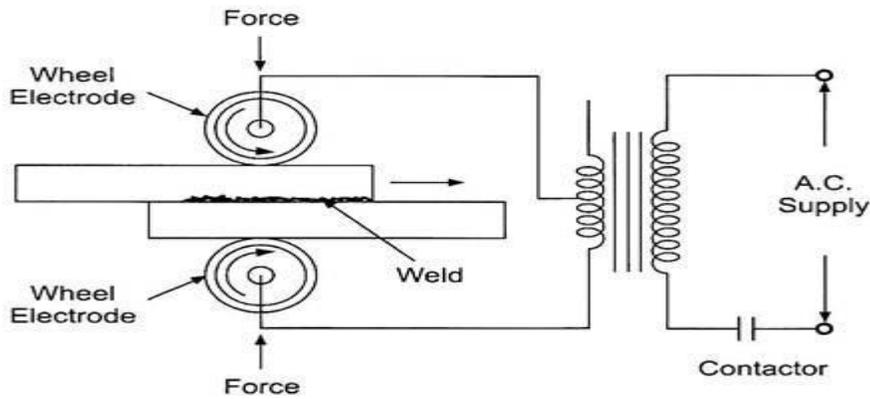
**Fig. 4.7** Principle of Seam Welding
