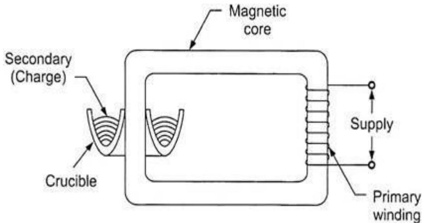
**Fig. 3.12** Core type furnace
