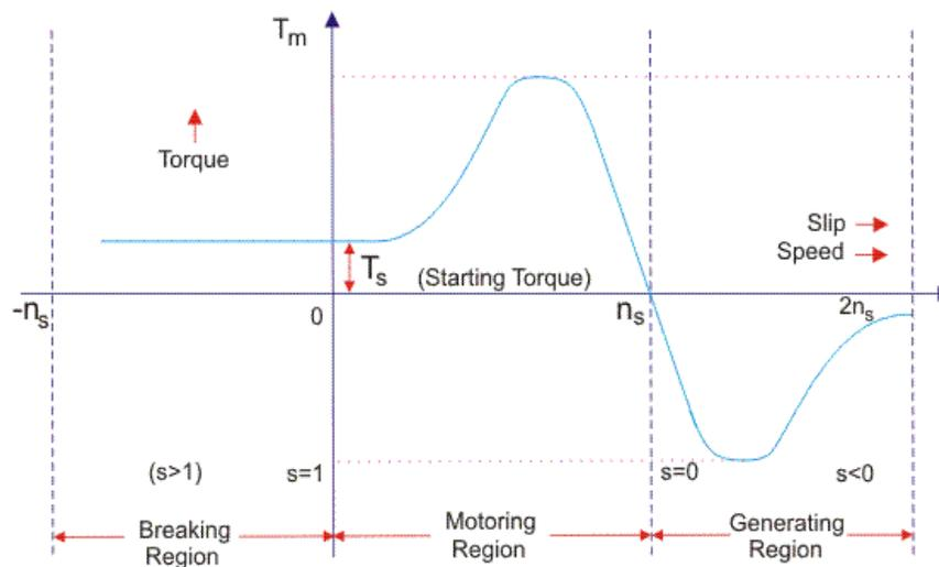
**Torque Slip Curve for Three Phase Induction Motor**
