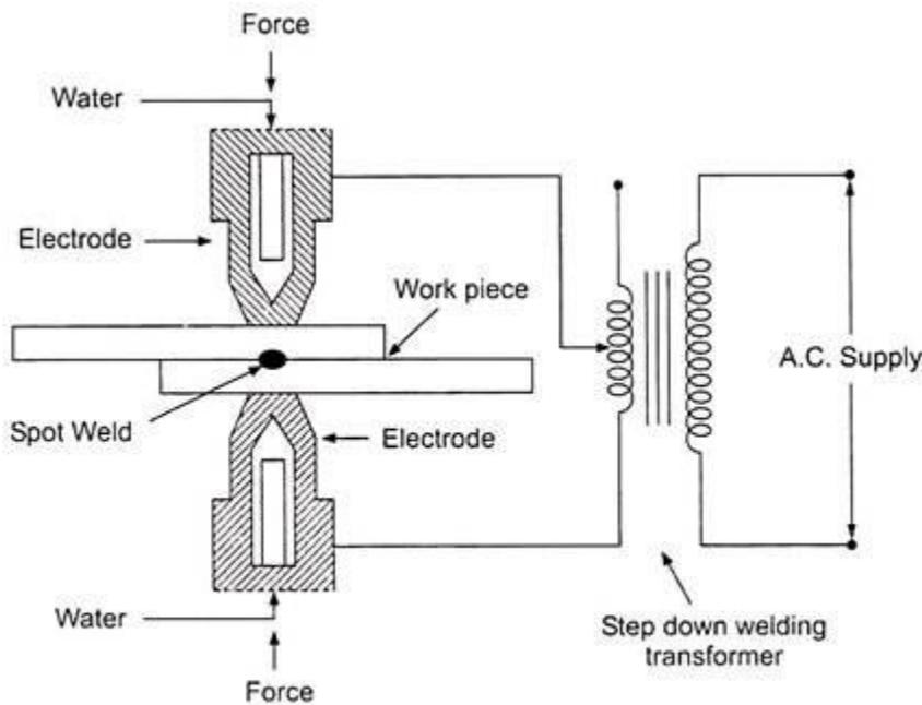
**Fig. 4.4** *Principle of Spot Welding*
