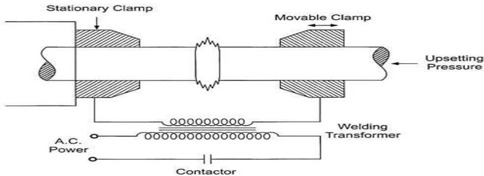
Fig. 4.9 Flash Butt Welding
