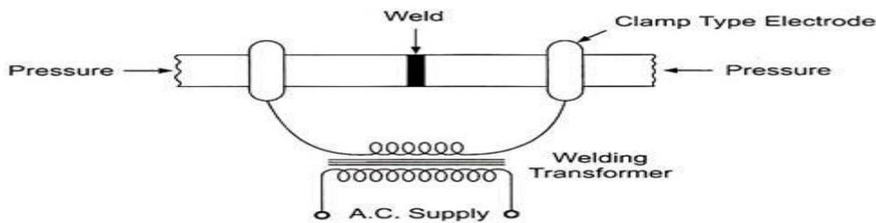
**Fig. 4.8** Butt Welding
