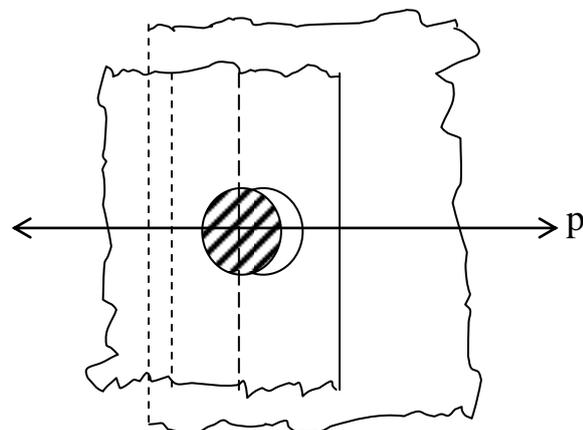
Crushing resistance  $P_C = n.d.t. \sigma_C$
