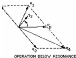
If the input frequency is greater than resonant frequency, the phase difference between  $v_1$  and  $v_3$  is less than  $90^\circ$ . Here  $V_{a1}$  is reduced and  $v_{a2}$  is increased. The phase difference between  $v_1$  and  $v_3$  is  $< 90^\circ$  and between  $v_2$  and  $v_3$  is  $> 90^\circ$ .
